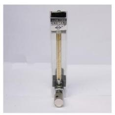
The main measuring components of the glass rotameter are a vertically mounted small upper and large tapered glass tube and a float that can be moved up and down. When the fluid passes through the conical glass tube
